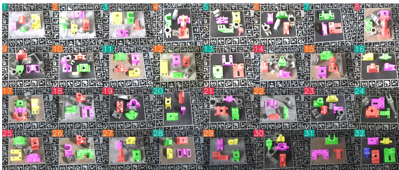
Fig. 2 Sample images of 32 scenes overlaid with colored 3D models with the ground truth poses (only target objects were overlaid). The number of each scene is shown in the upper left corner, and the color
